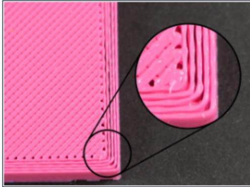
Under-Extrusion
