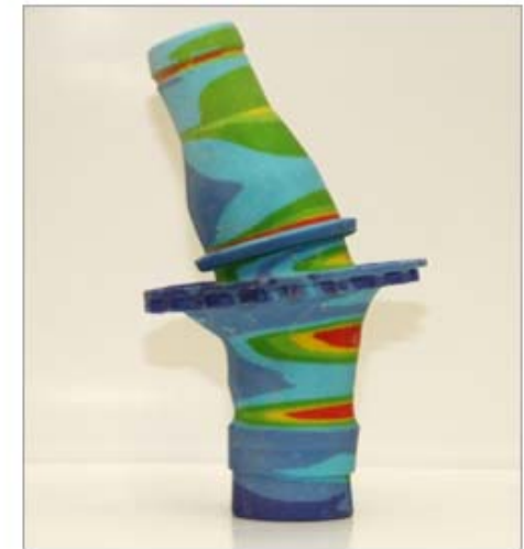
Finite Element Result - Corvette GT2 Spindle Stress Colored and Deformation x1000
